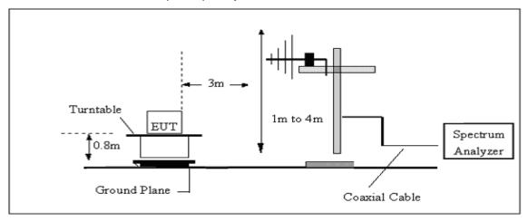
(B) Radiated Emission Test-Up Frequency Above 1GHz
