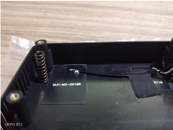
WIFI main antenna
