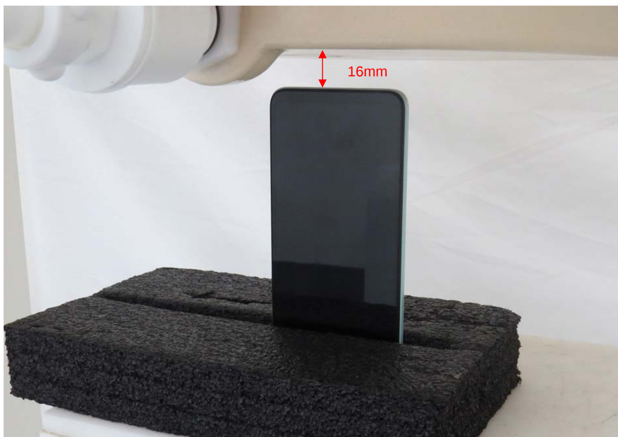
Picture 20: Bottom Edge, the distance from handset to the bottom of the Phantom is 16mm
