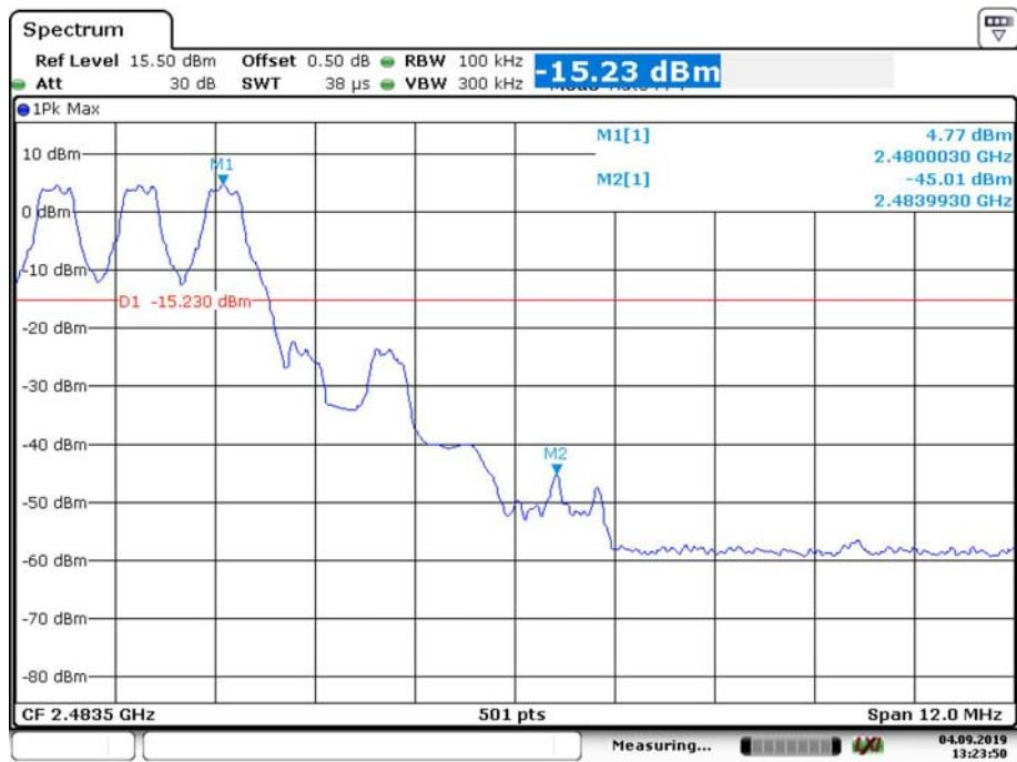
*EDR Mode ( $\pi/4$ -DQPSK):***Band Edge, Left Side**
