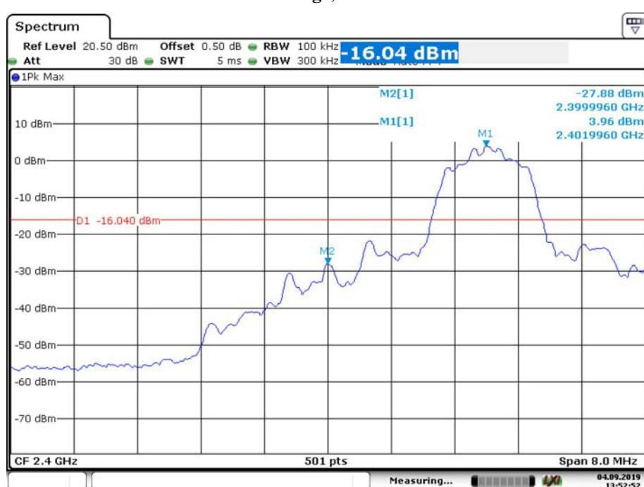
**Band Edge, Right Side**
