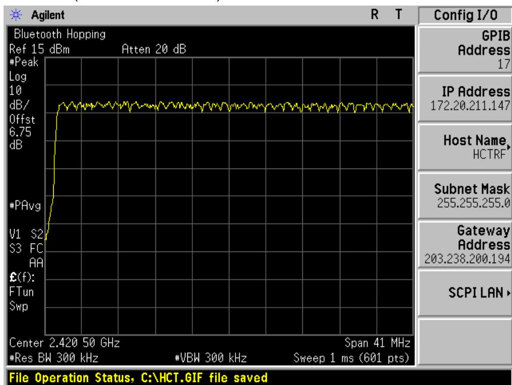
Number of Channels (2.441 GHz - 2.4835 GHz) 8DPSK
