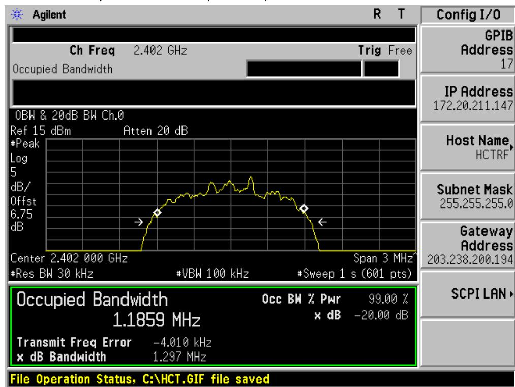
20 dB Bandwidth & Occupied Bandwidth (Mid-CH) 8DPSK
