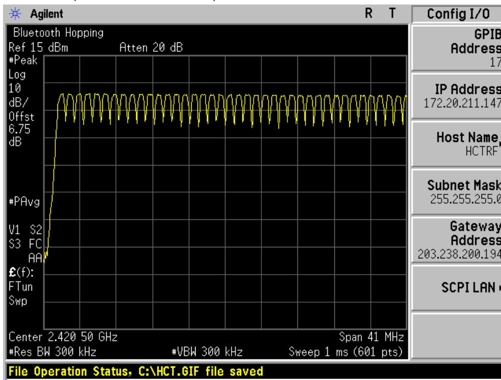
Number of Channels (2.441 GHz - 2.4835 GHz) GFSK
