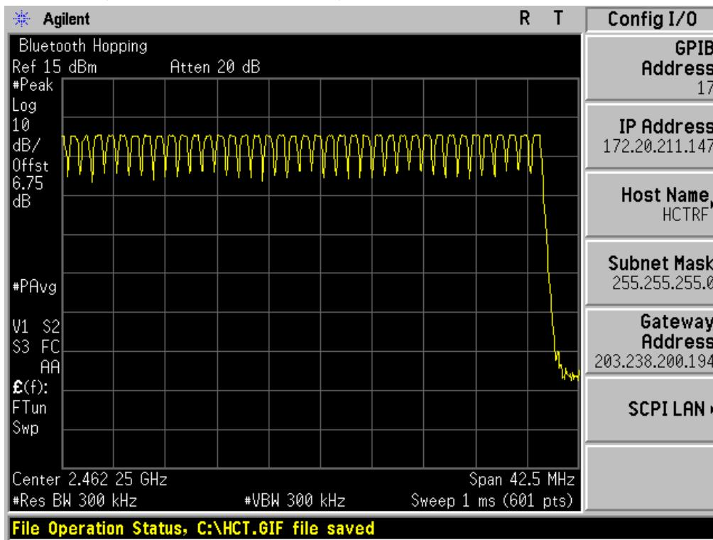
Number of Channels (2.4 GHz - 2.441 GHz) 8DPSK
