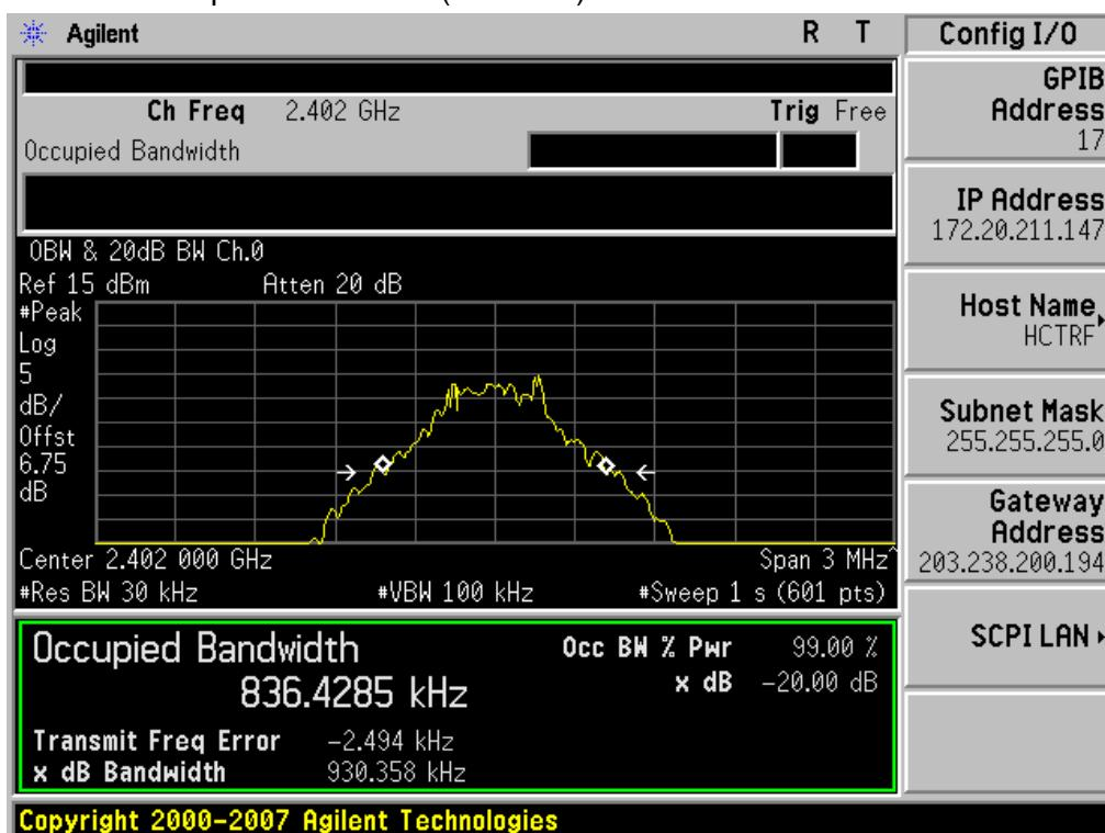
20 dB Bandwidth & Occupied Bandwidth (Mid-CH) GFSK
