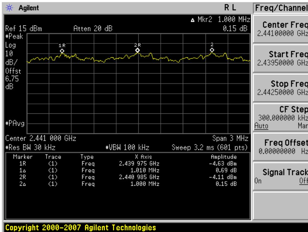
Channel Separation ( $\pi/4$ DQPSK)
