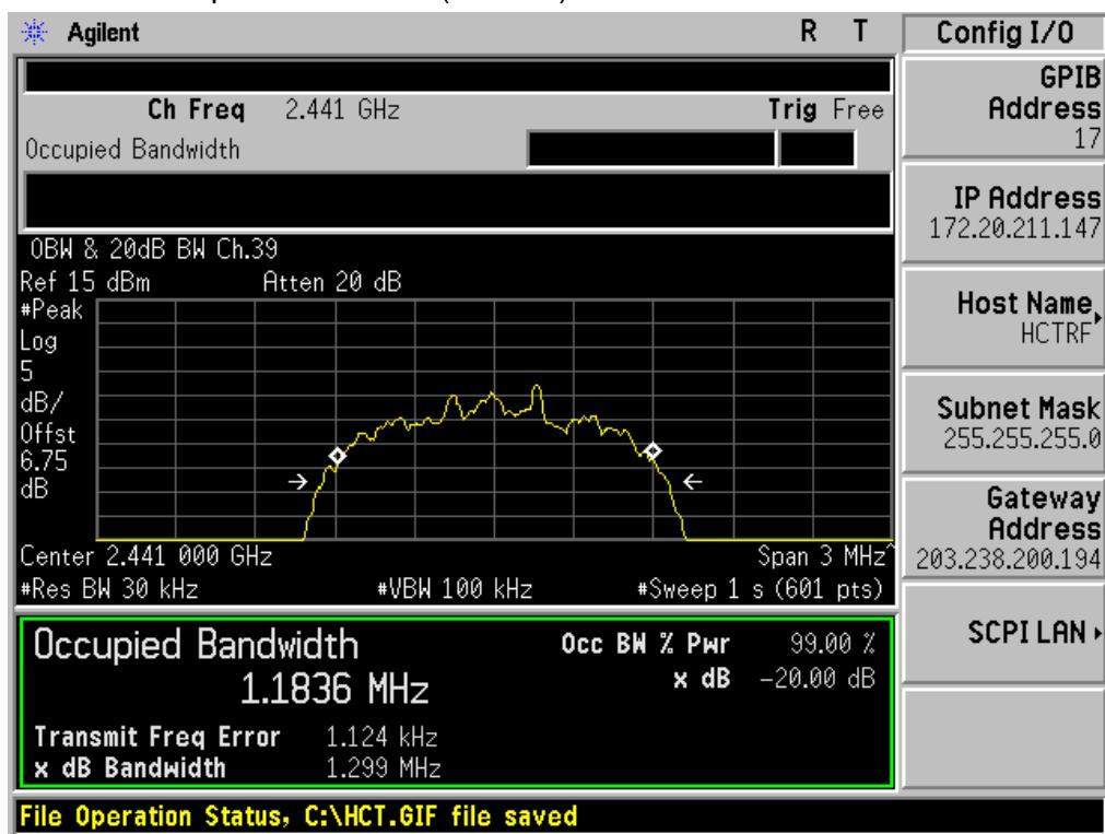
20 dB Bandwidth & Occupied Bandwidth (High-CH) 8DPSK
