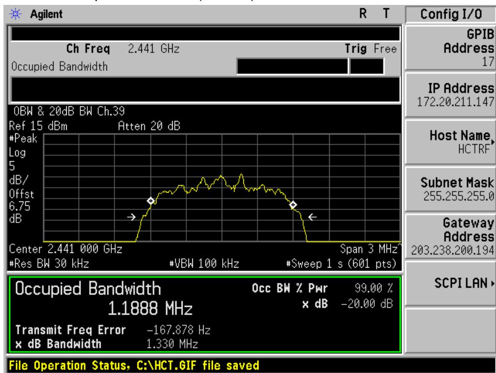
20 dB Bandwidth & Occupied Bandwidth (High-CH)  $\pi/4$ DQPSK
