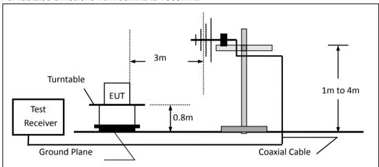
(c) For radiated emissions above 1000MHz
