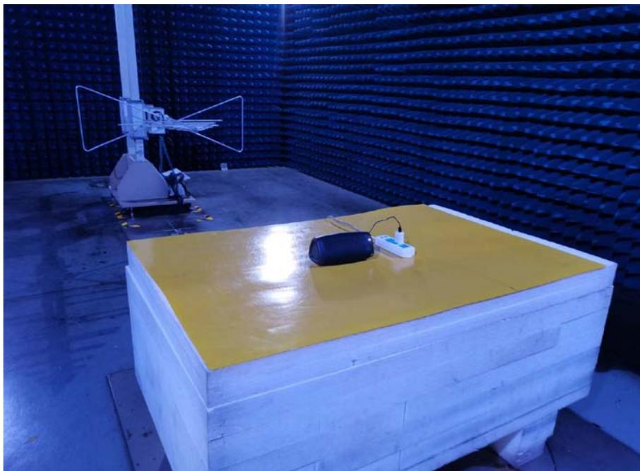
**Radiated Spurious Emissions Test View (Above 1GHz)**
