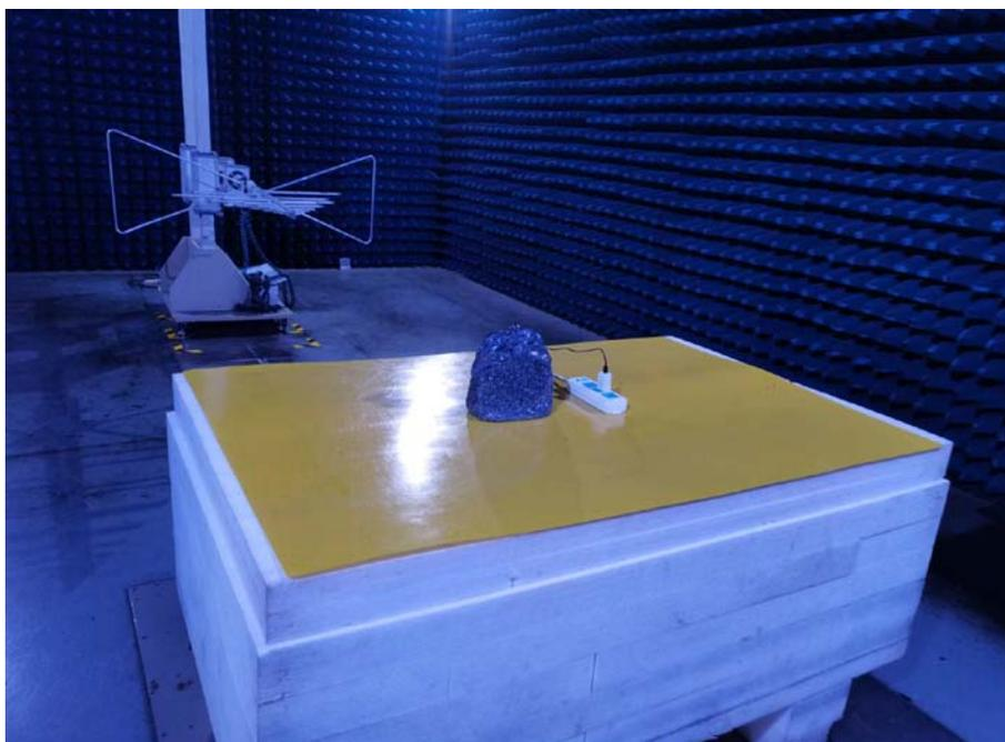
**Radiated Spurious Emissions Test View (Above 1GHz)**
