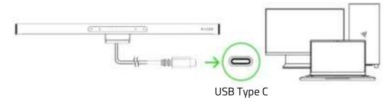
i For optimal performance, make sure to connect the light bar to the USB Type C port of your PC directly.
