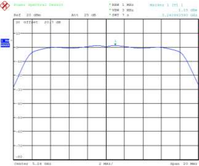
Figure 5-2: Peak Power Spectral Density 802.11a, Channel 48, 6 Mbps
