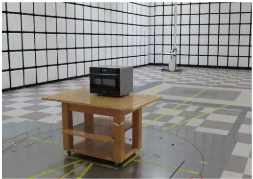
Radiated Test Picture : 30 Mb ~ 1 Gb (Front)
