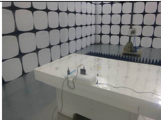
Radiated Spurious Emissions Test Setup Above 1GHz
