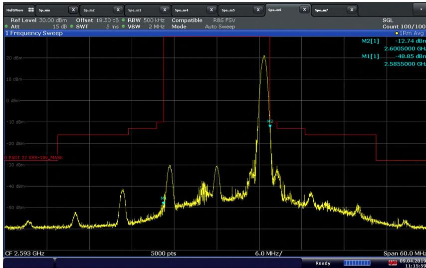
LTE Band 41 (20 MHz BW)/QPSK/Middle Channel 2593 MHz
