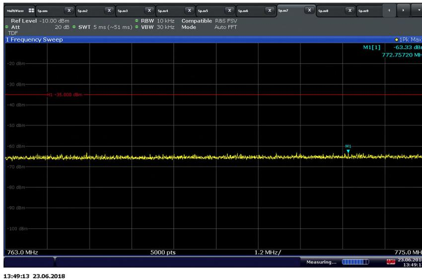
LTE Band 13 (5 MHz BW)/QPSK/Middle Channel 782 MHz Conducted Spurious Emissions (793-806 MHz)
