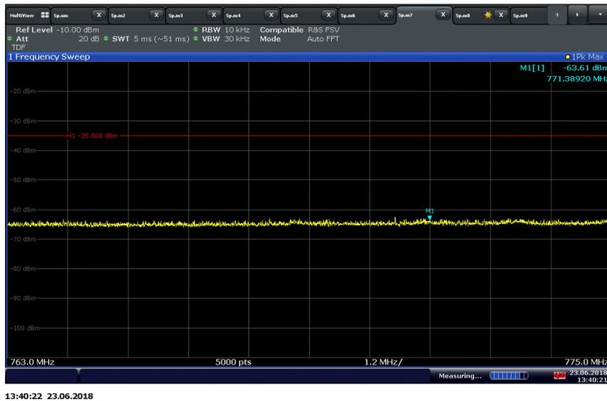
LTE Band 13 (10 MHz BW)/QPSK/Middle Channel 782 MHz Conducted Spurious Emissions (793-806 MHz)
