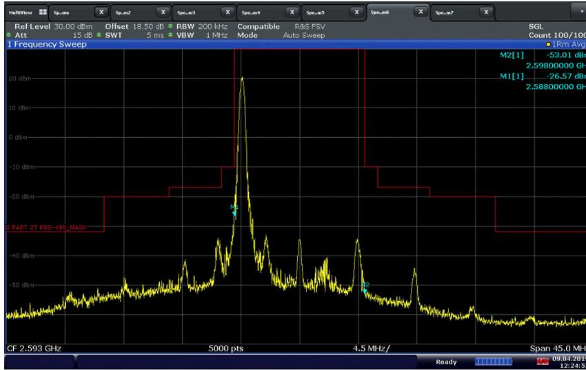
LTE Band 41 (10 MHz BW)/QPSK/Middle Channel 2593 MHz 1RB 49 offset Mask
