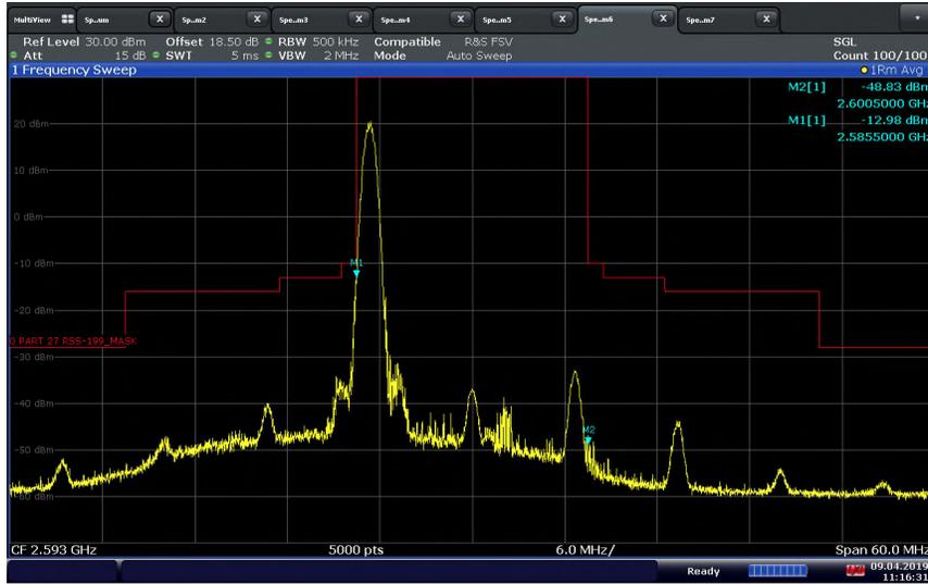
LTE Band 41 (15 MHz BW)/QPSK/Middle Channel 2593 MHz 1RB 74 offset Mask
