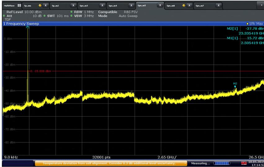
LTE Band 41C\_10 MHz BW\_2585.9 MHz 1RB49 + 15 MHz BW\_2597.9 MHz 1RB0 /QPSK
