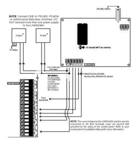
**CAUTION**: Due to the sensitivity of the RF circuitry, avoid any contact with the coils and potentiometers on the LINKS2450 circuit board.
