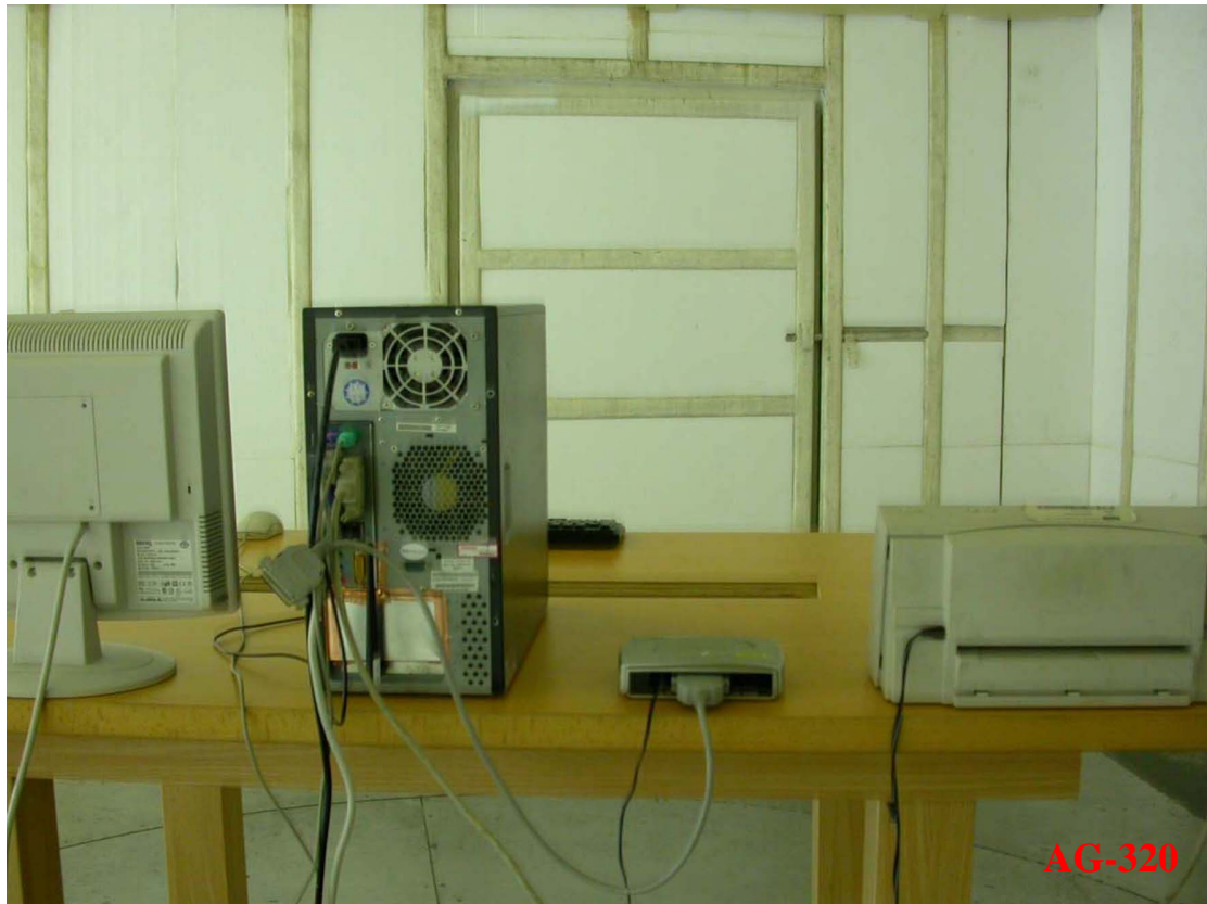
Photo 1: Radiated Emission Test set-up photo
