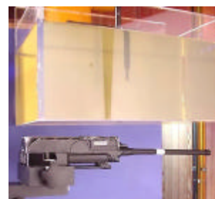
Face-held SAR Test Setup 2.5cm Separation Distance
