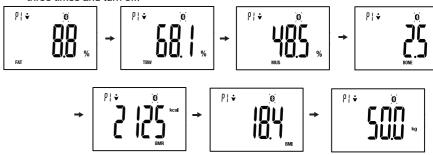
• If it identifies two or more users,for example,P1,P2 and P3, the LCD will display these users altermately two times, you may press the function key ▲ or ▼ to choose the User ID. The measuring results will then be stored into the User ID you selected and displayed sequentially three times. If you don't choose the user, it will turn off.
