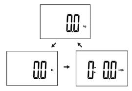
Note: If there is no operation in the weighing mode, the scale will turn off after a few seconds.
