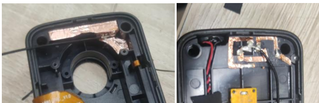
Location of wifi antenna Wireless microphone antenna position
