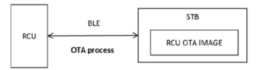
From diagram above, the STB can transfer the RCU firmware by the BLE link.
