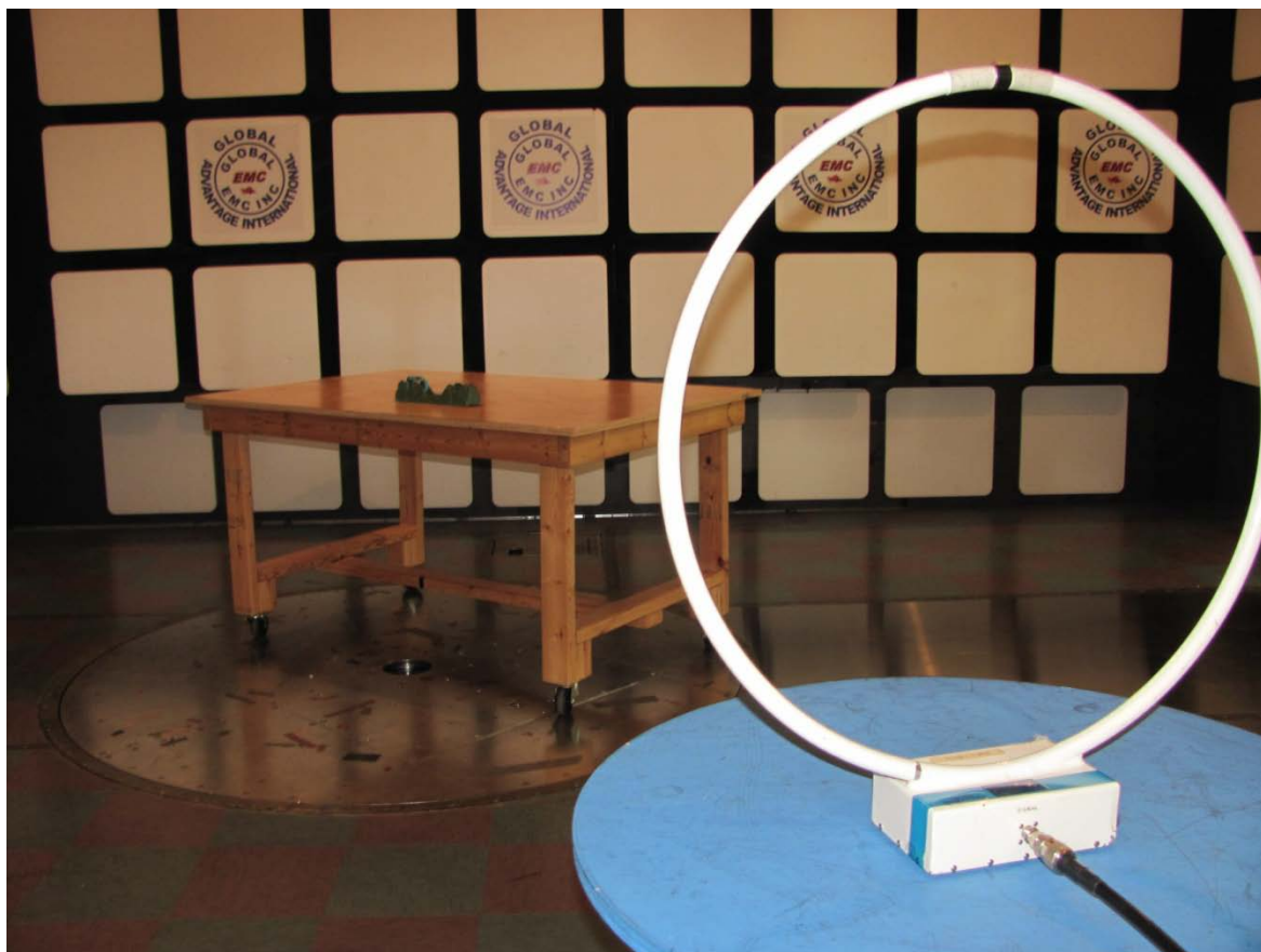
Illustration 1: Radiated emission setup – photo 1
