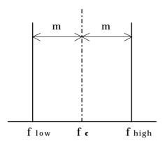
The peak-to-peak deviation of the FSK signal is approximately 3.6 KHz ("sliver modulation")
