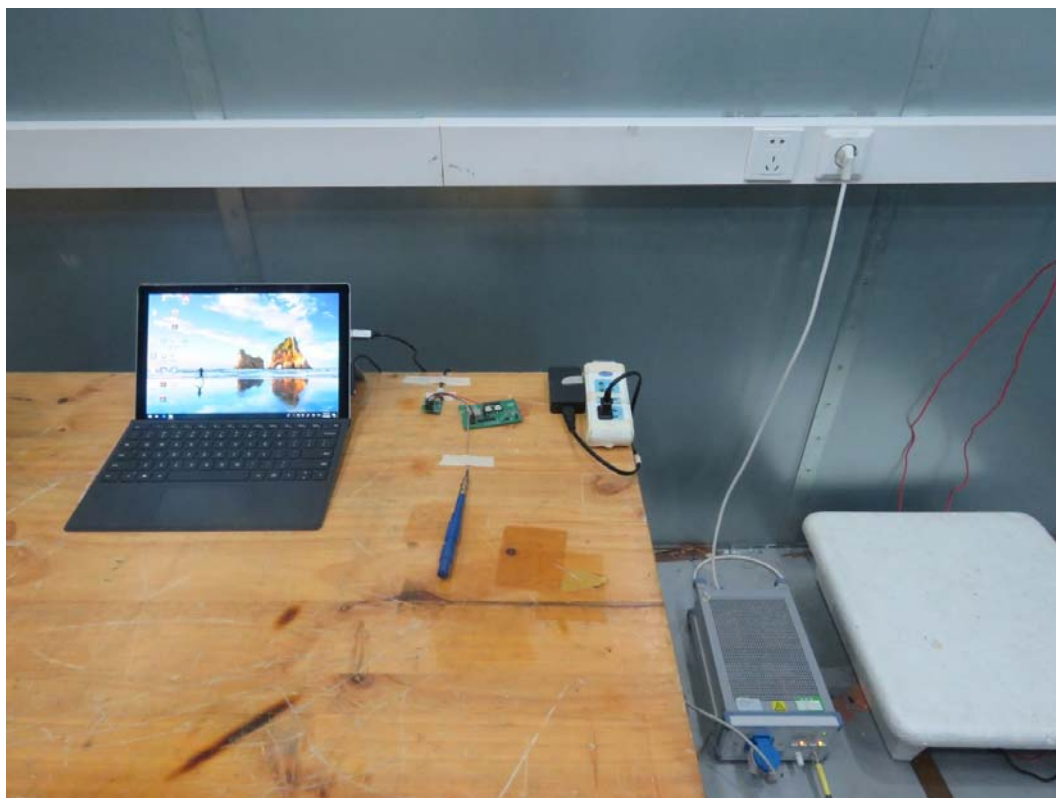
Picture 2 Conducted Emission Test Setup
