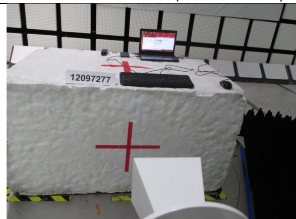
RADIATED FRONT PHOTO (ABOVE 18-40 GHz)
