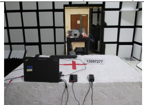
RADIATED BACK PHOTO (ABOVE 18-40 GHz)
