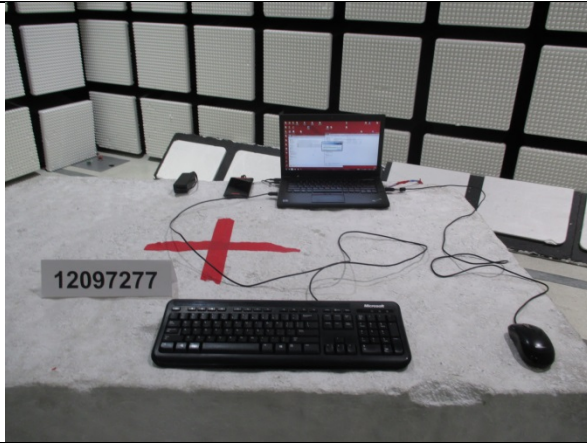
RADIATED FRONT PHOTO (BELOW 1 GHz)
