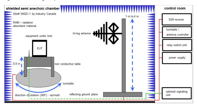
Measurement distance: tri-log antenna 10 meter
