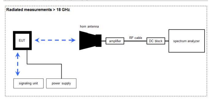
Measurement distance: horn antenna 50 cm
