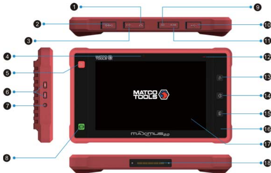
Fig. 2-4 MAXIMUS2.0 Display Tablet (front & side view)
