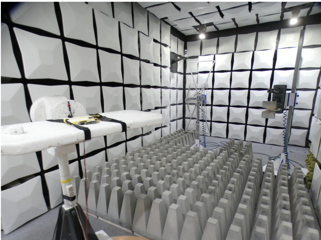
Photo 4: Test setup for radiated measurements above 1 GHz
