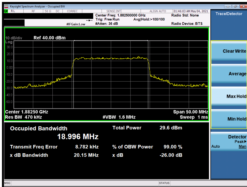
Plot 7-44. Occupied Bandwidth Plot (NR Band n25/2 - 20.0MHz CP-OFDM QPSK - Full RB)
