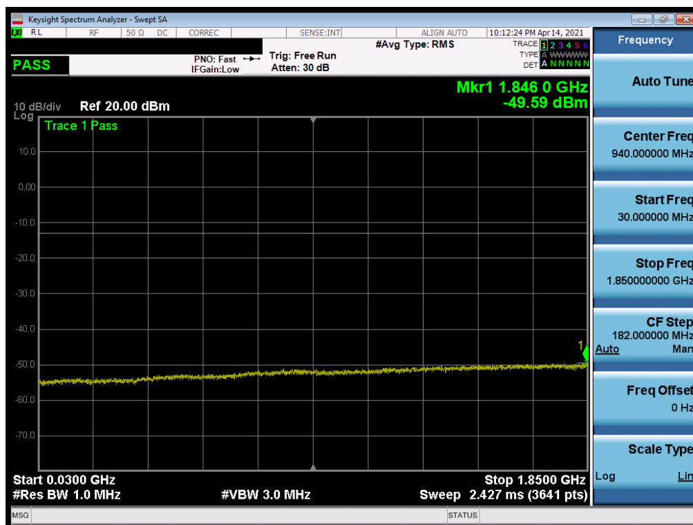
Plot 7-98. Conducted Spurious Plot (WCDMA Ch. 9400)
