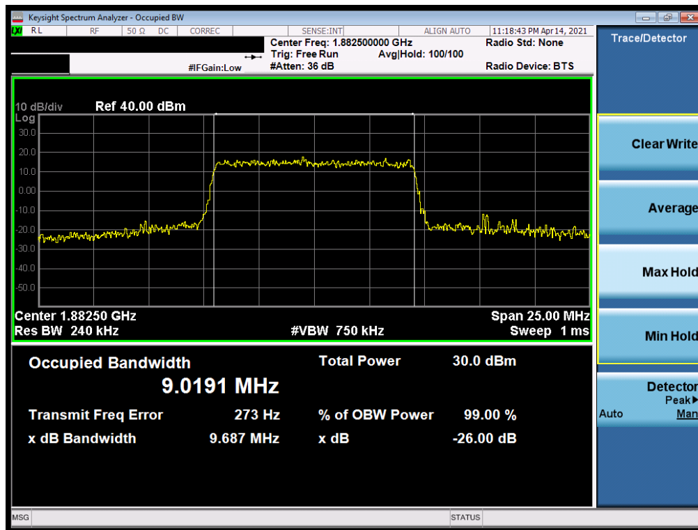
Plot 7-5. Occupied Bandwidth Plot (LTE Band 25/2 - 10MHz QPSK - Full R
