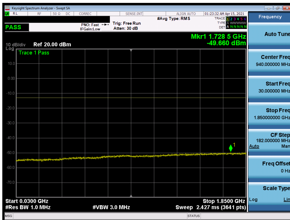
Plot 7-107. Conducted Spurious Plot (CDMA Ch. 600)
