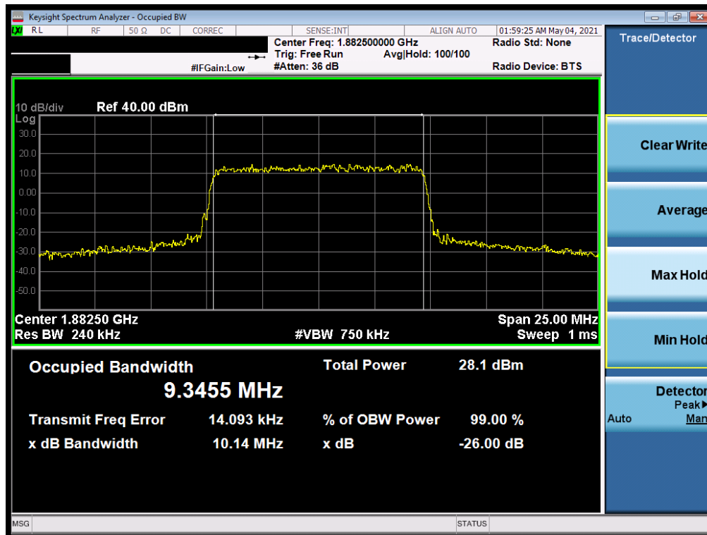
Plot 7-51. Occupied Bandwidth Plot (NR Band n25/2 - 10.0MHz CP-OFDM 16QAM - Full RB)
