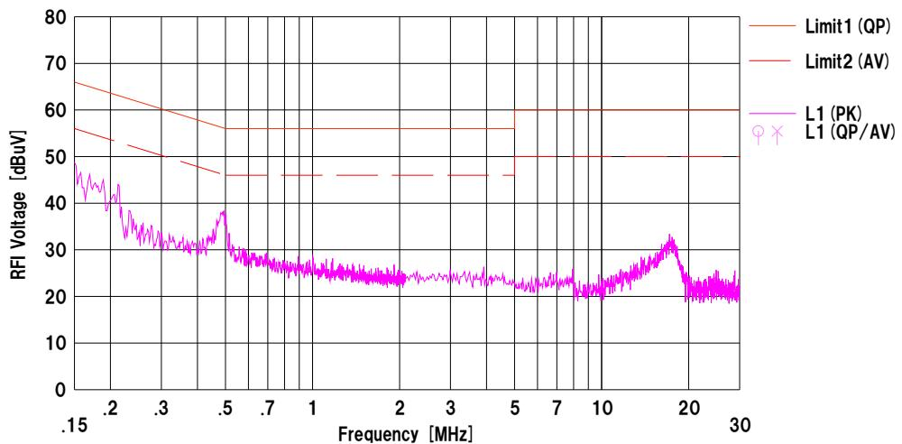
Calculation:Result [dBuV] =Reading [dBuV] +C.Fac (LISN (AMN) +Cable+ATT) [dB]
