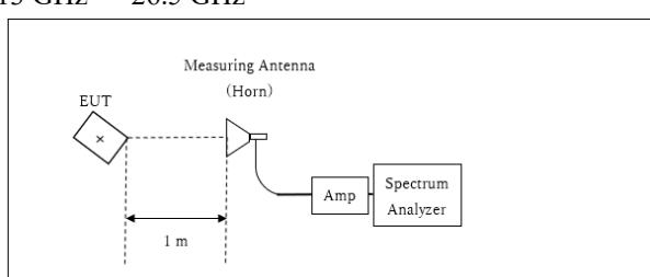
Distance Factor:  $20 \times \log (1.0 \text{ m}^* / 3.0 \text{ m}) = -9.54 \text{ dB}$
