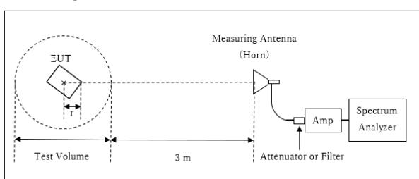
Distance Factor:  $20 \times \log (3.85 \text{ m}^*/3.0 \text{ m}) = 2.17 \text{ dB}$
