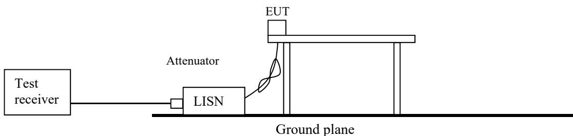
The AC Mains Terminal Continuous disturbance Voltage has been measured with the EUT in a shielded room. The EUT was connected to a LISN (AMN).
