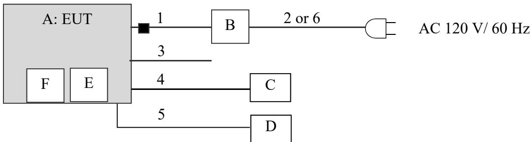
\* Cabling and setup(s) were taken into consideration and test data was taken under worse case conditions.
