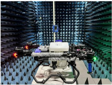
RF Radiated Test (18-40GHz)
