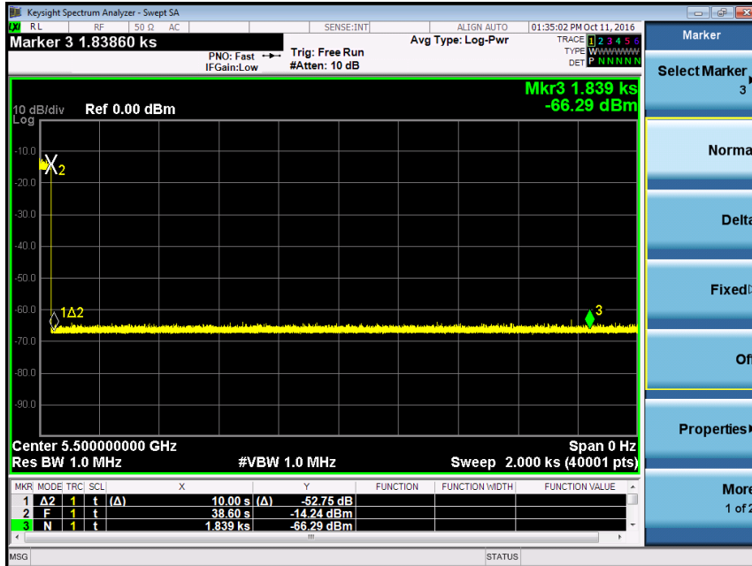
5510 MHz - 2000 sec Timing Plot
