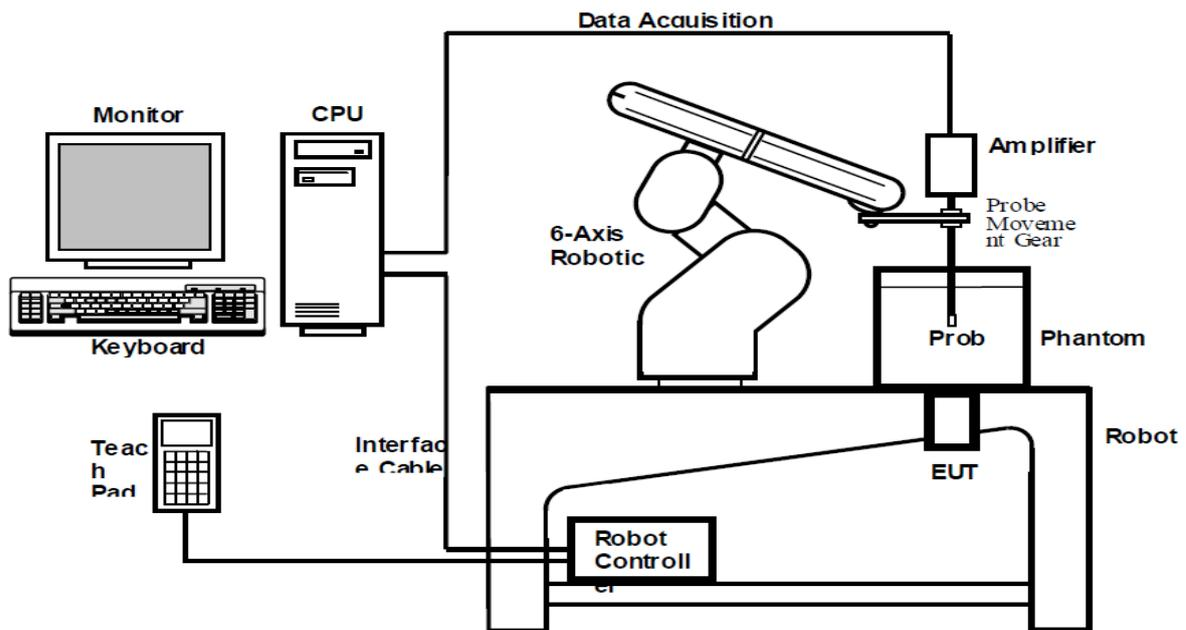
The system is remote controlled by a PC, which contains the software to control the robot and data acquisition equipment. The software also displays the data obtained from test scans by calculating the measured values into corresponding SAR values based on the currently acceptable calculation methods.
