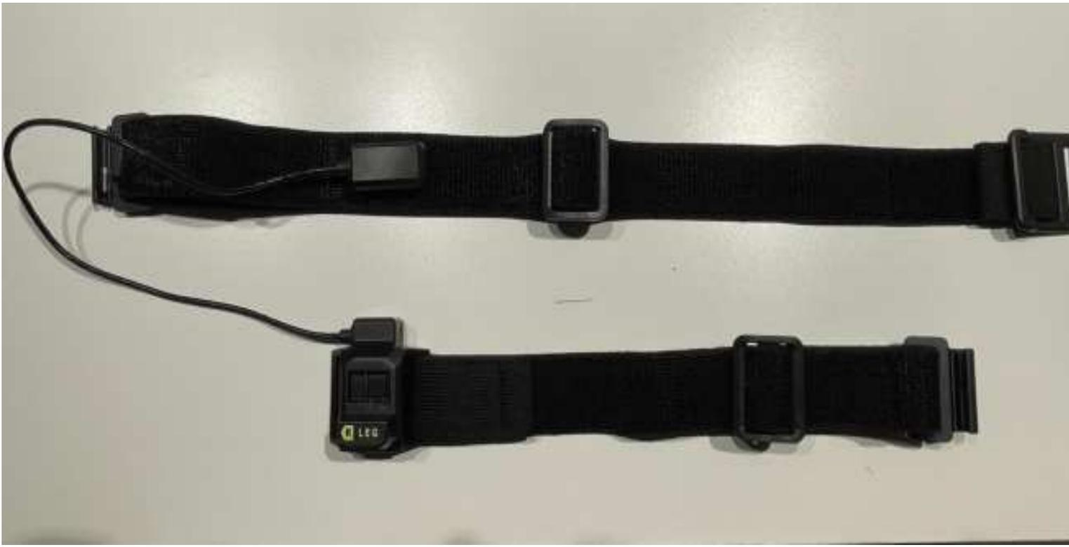
4. Attach the cable fixing strap to the cord connecting the knee sensor and the leg sensor.
