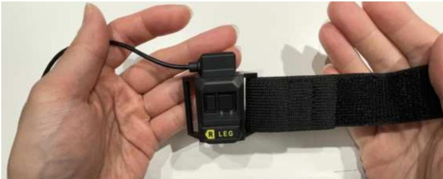
3. Attach the Left and Right knee sensors to the middle length straps (Knee straps).
