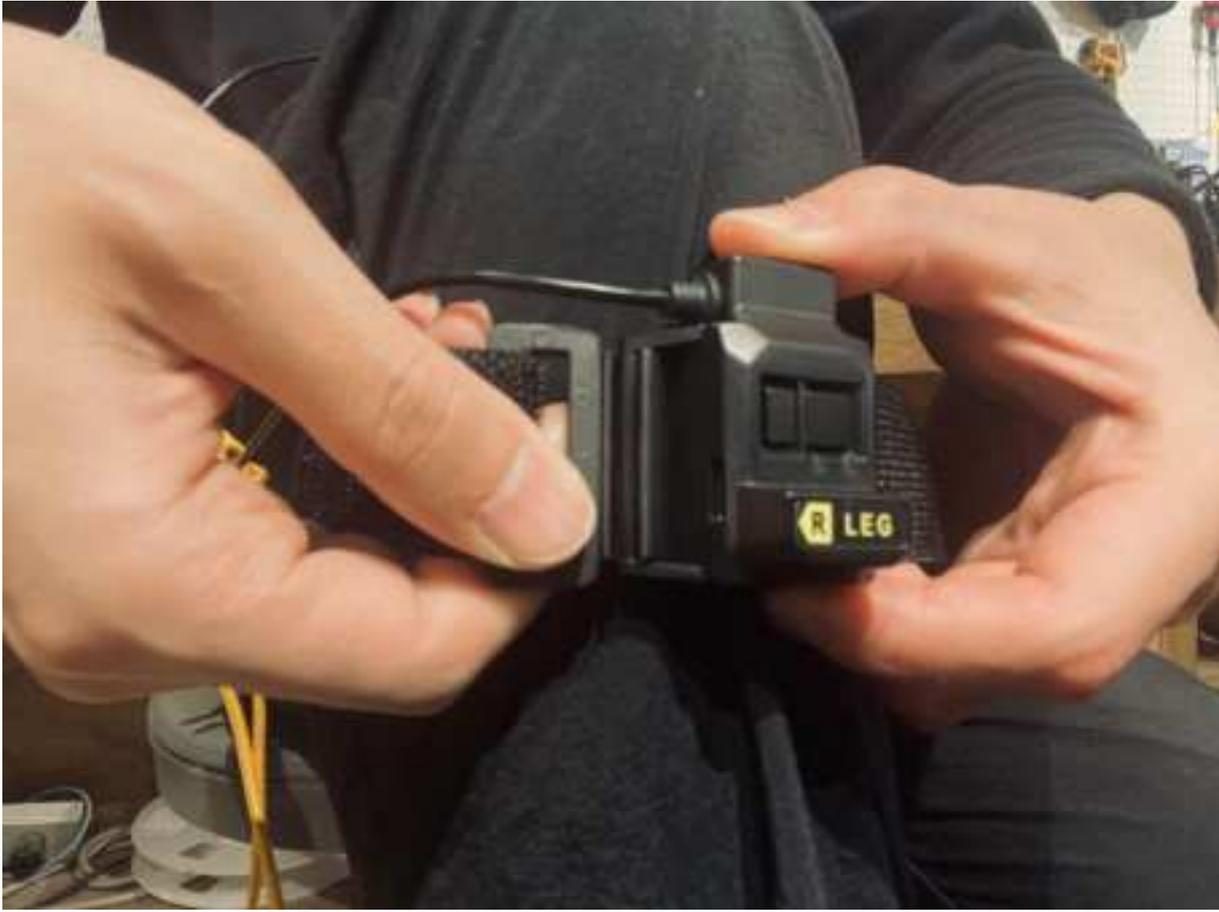
*You can attach the knee sensors anywhere between the thigh and the knee. Choose a position where the strap is less likely to slip, depending on your body type. As with the previous instructions, ensure the height is aligned on both sides.*
