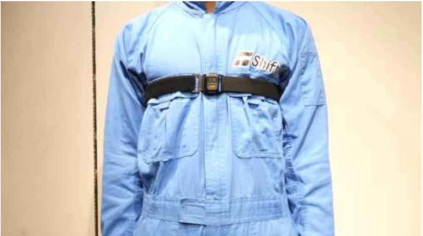
*Place the chest sensor as high as possible, and the hip sensor as close to the pelvis as possible.*
