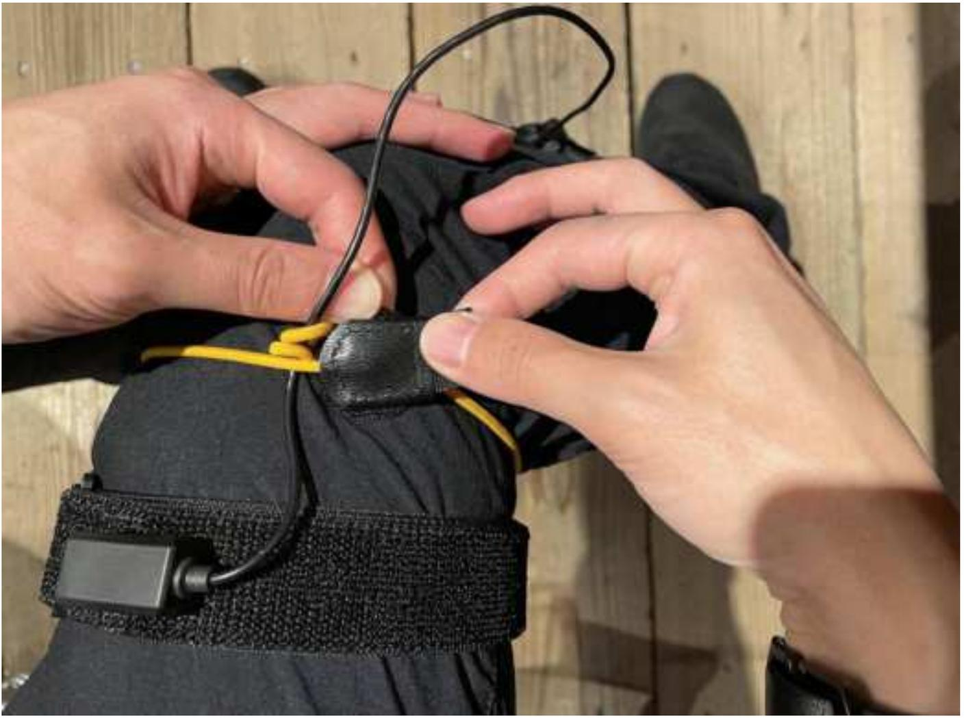
*\*The leg sensors have a distance sensor to detect the movement of the ankle.
