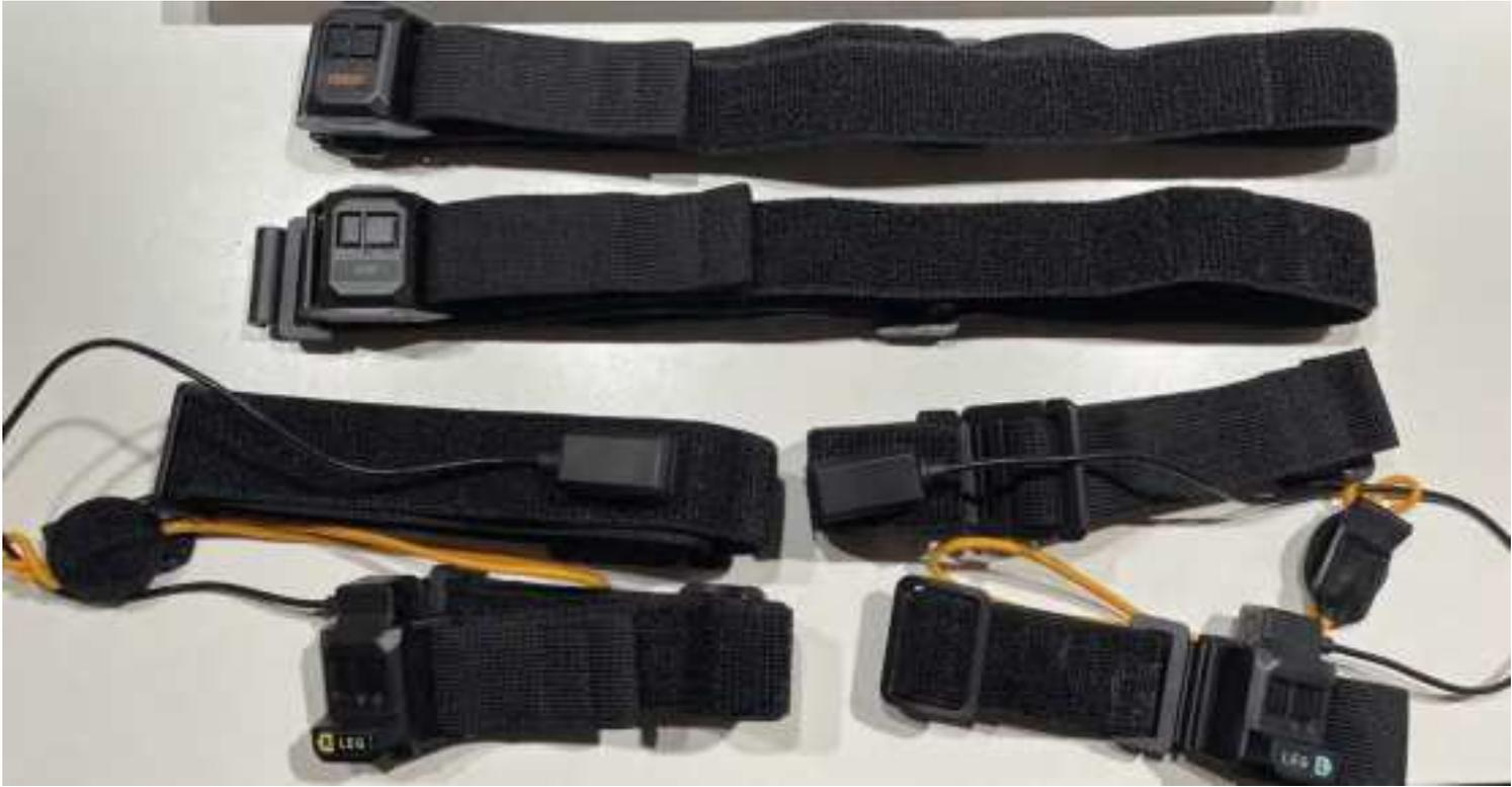
*2. Put each sensor on your body. Ensure the sensor is positioned correctly and oriented vertically. Note that it will not function properly if placed in the wrong position or direction.*
