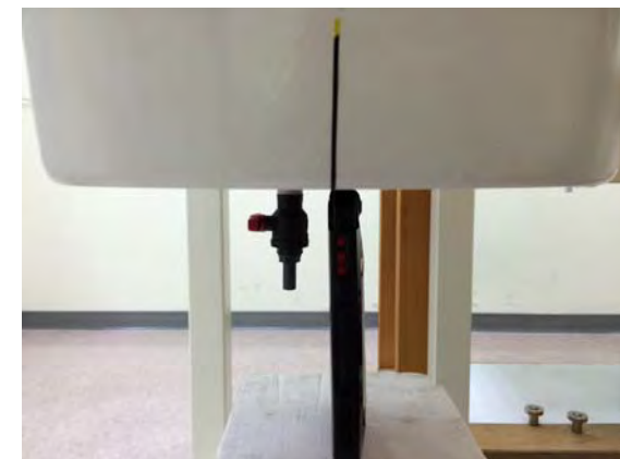
Fig.5 EUT Right side to flat phantom
