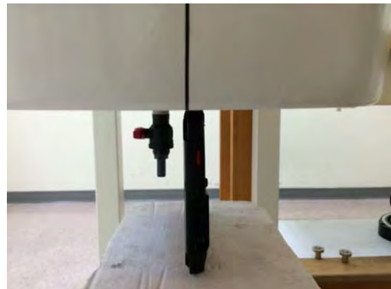
Fig.6 EUT Top side to flat phantom
