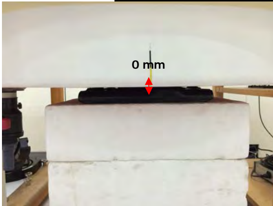
Fig.3 EUT Back side to flat phantom
