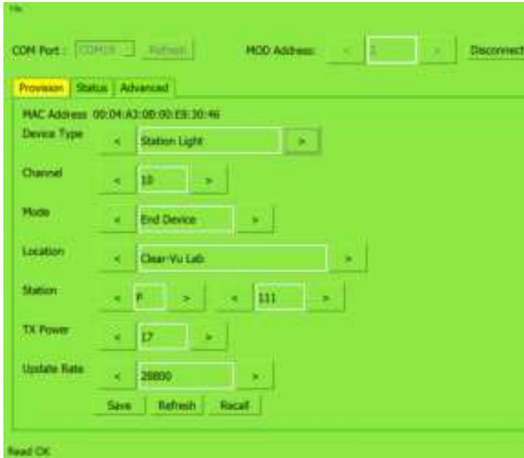
Figure 8: Provision Tab Window (Station Configuration)
