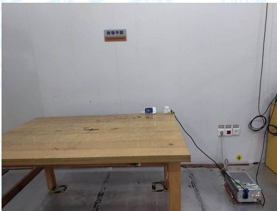
Photo of Setup for Conducted Emission
