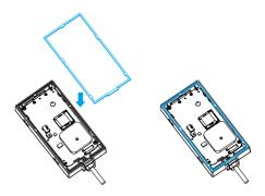
5. Press the upper case down and make sure all 5 clips are completely in place.
