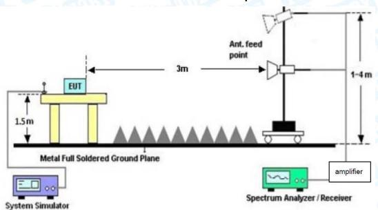
**Above 1GHz Test Setup**
