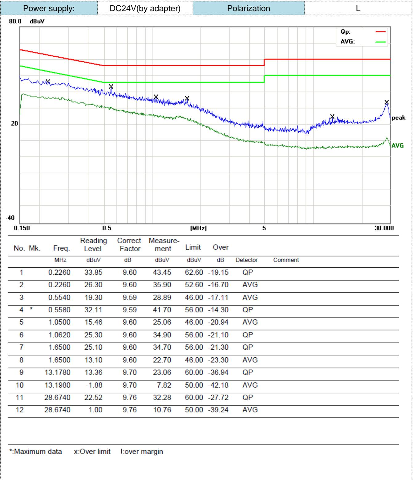
Power supply: DC24V(by adapter) Polarization N
