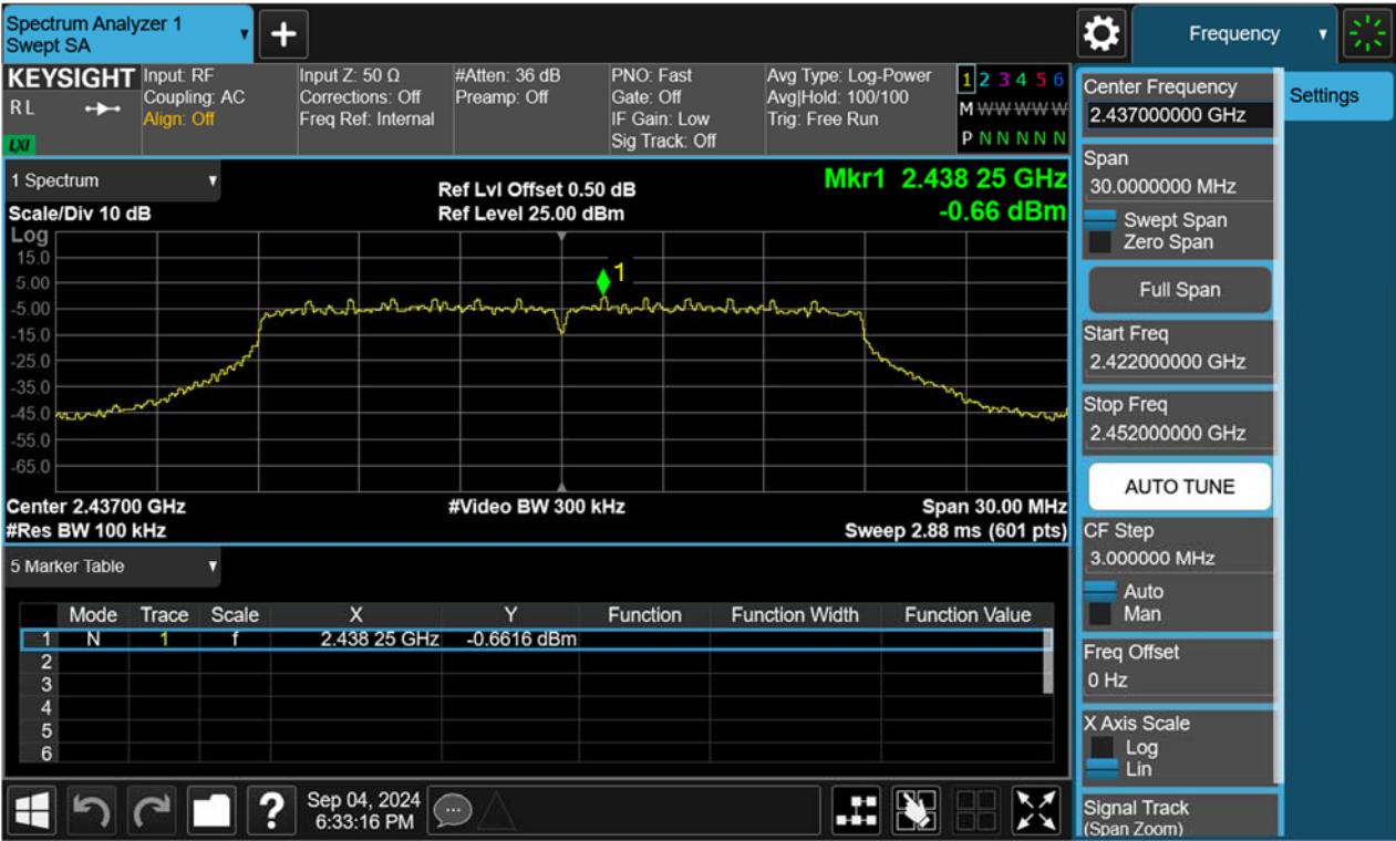
Conducted spurious emissions 30MHz-25GHz
