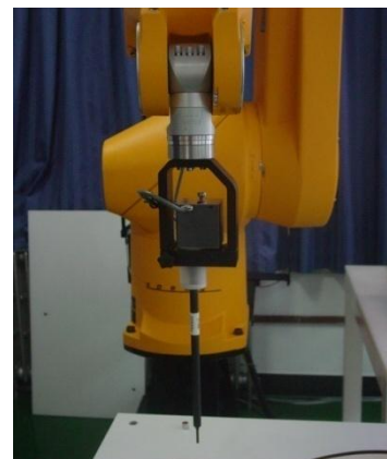
Picture C.3 E-field Probe
