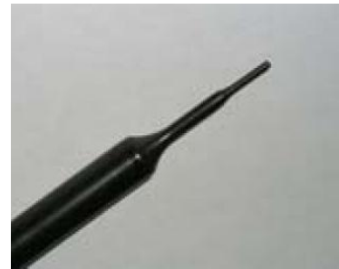
Picture C.2 Near-field Probe
