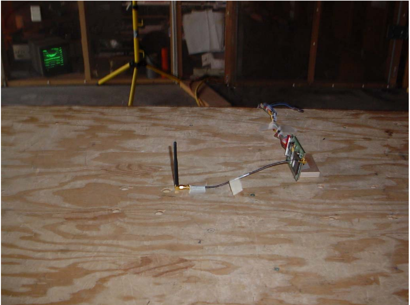
Radiated Emissions @ 3 Meters EUT with Quarter Wave Antenna, 1.5 dBi Gain
