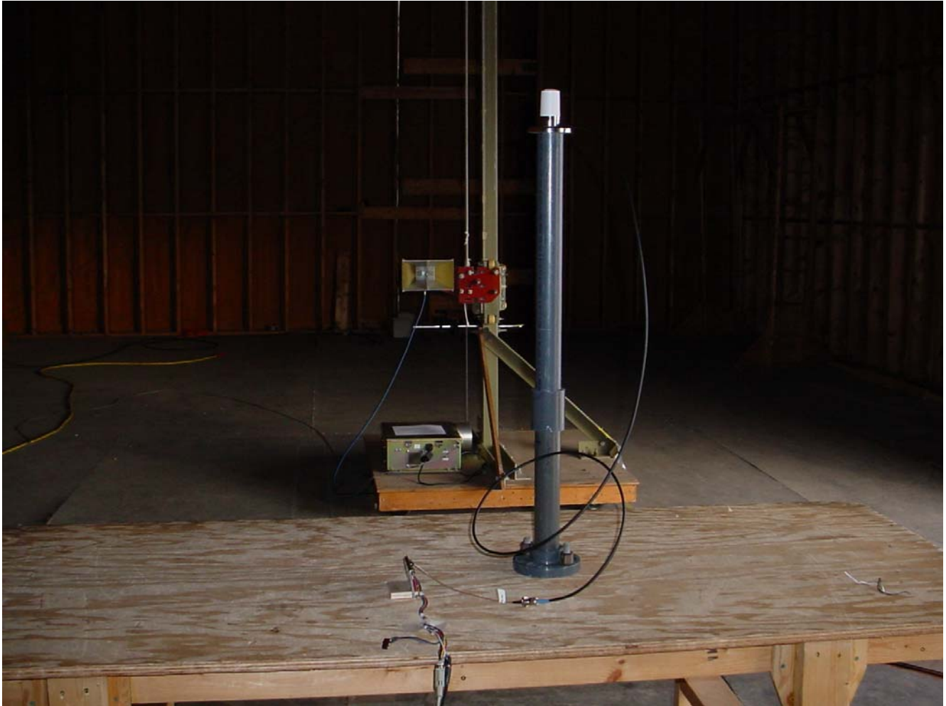
Radiated Emissions @ 3 Meters EUT with Transit Antenna, 5.15 dBi Gain
