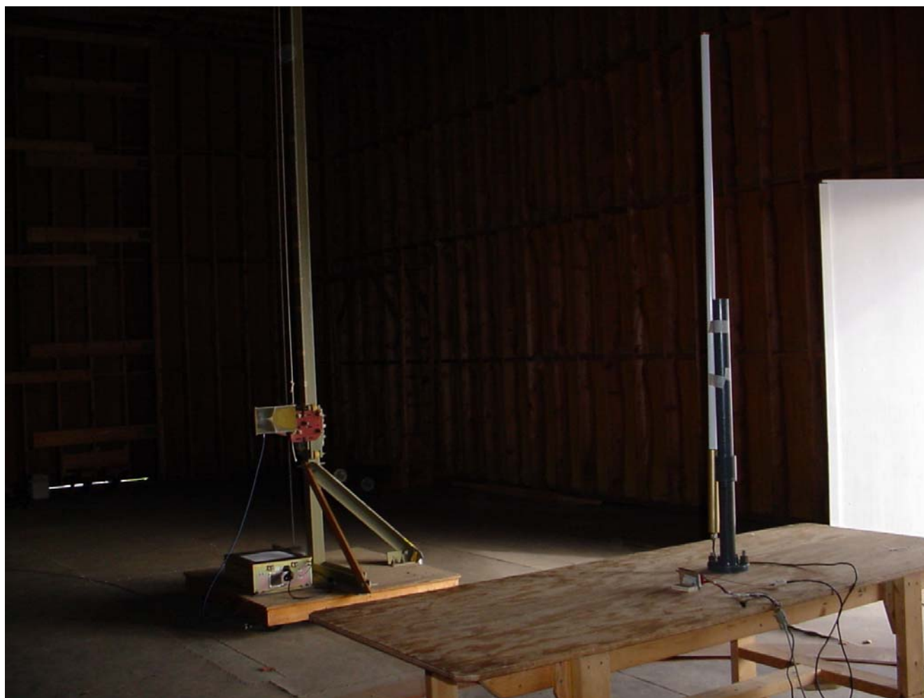
Radiated Emissions @ 3 Meters EUT with Omni Directional Antenna, 8.15 dBi Gain
