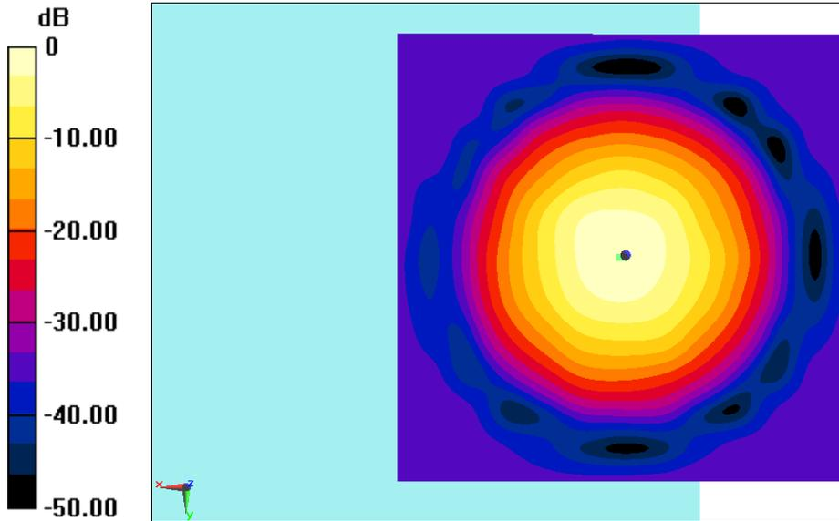
$0 \text{ dB} = 0.6909 \text{ A/m} = -3.21 \text{ dBA/m}$ **Fig B.2 T-Coil GSM 850**
