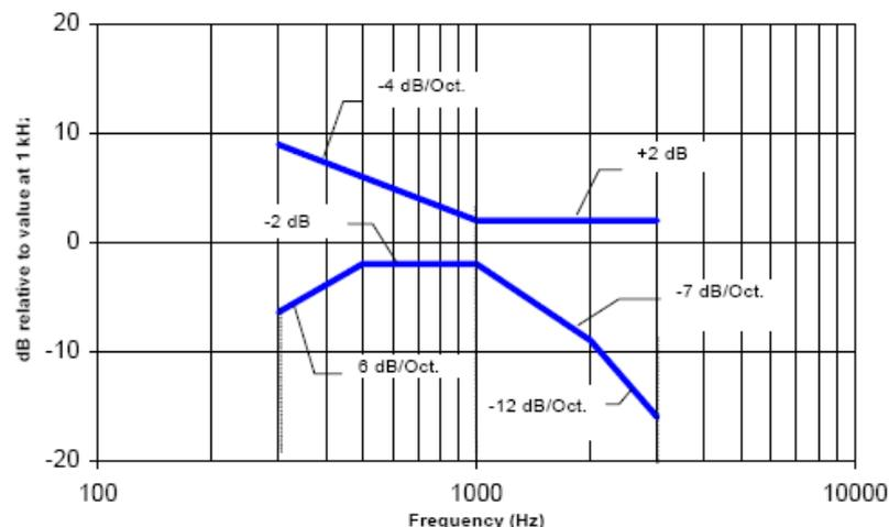
NOTE—Frequency response is between 300 Hz and 3000 Hz.
