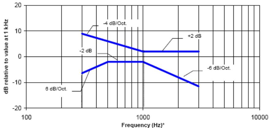
NOTE—Frequency response is between 300 Hz and 3000 Hz.
