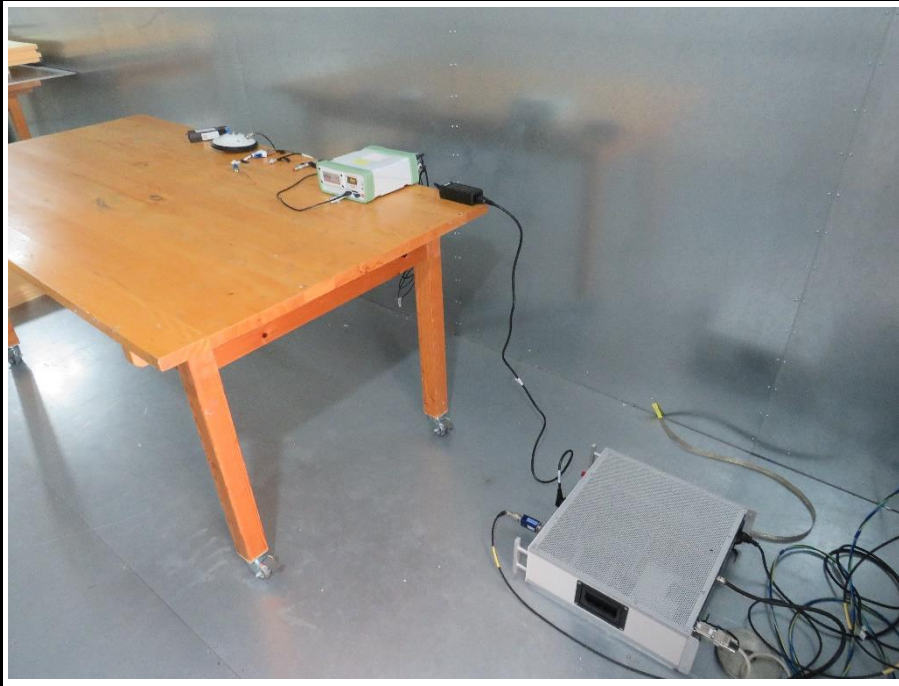
Setup for measurements 150 kHz – 30 MHz (with AC/DC Adapter)
