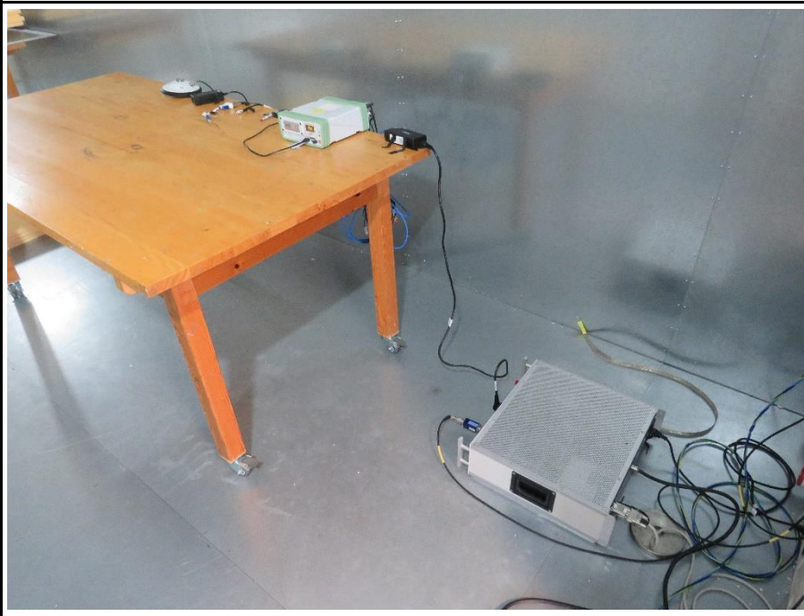
Setup for measurements 150 kHz – 30 MHz (with PoE)
