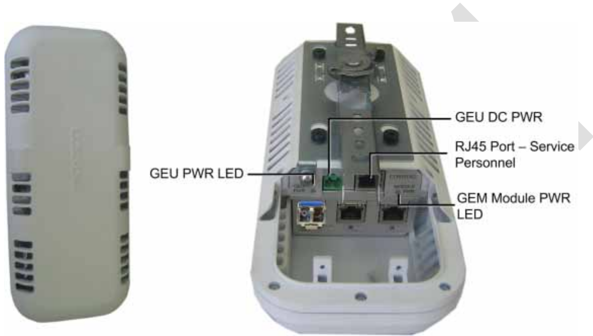
Figure 3-8. GEU Enclosure: Top (Left) and Open Underside (Right)
