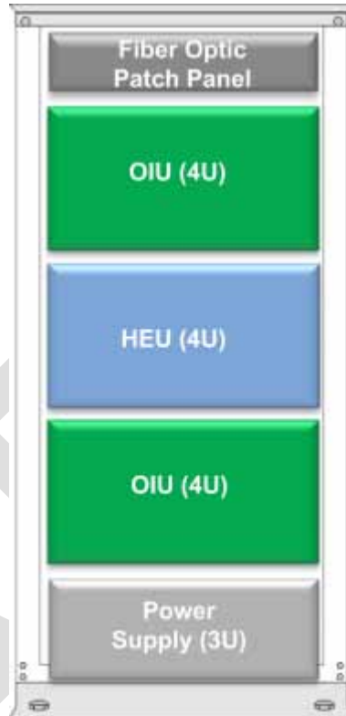
Figure 4-1. Example of Communication Rack Installation
