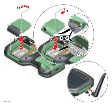
When the expansion cover or expansion pack are detached from the field controller, the IP68 protection does not apply! Look for a dry and dust free atmosphere when detaching the expansion cover or the expansion pack.
