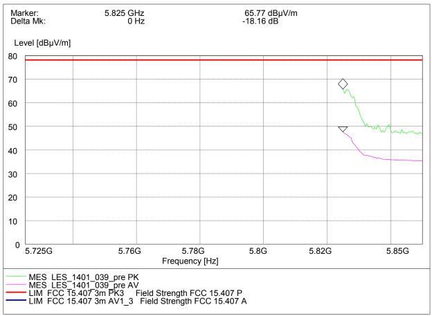
WLAN n-Mode, 20 MHz, 72.2 Mbit/s, CH 161, 5805 MHz
