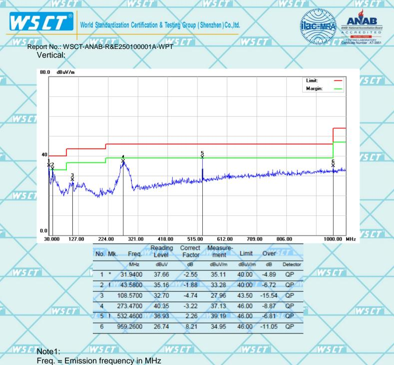
Freq. = Emission frequency in MHz Reading level  $(dB\mu V)$  = Receiver reading Corr. Factor (dB) = Antenna factor + Cable loss - Amplifier factor. Measurement  $(dB\mu V)$  = Reading level  $(dB\mu V)$  + Corr. Factor (dB)Limit  $(dB\mu V)$  = Limit stated in standard Margin (dB) = Measurement  $(dB\mu V)$  – Limits  $(dB\mu V)$
