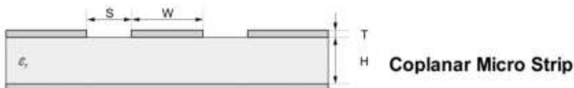
Figure 23: Coplanar micro-strip dimension specification
