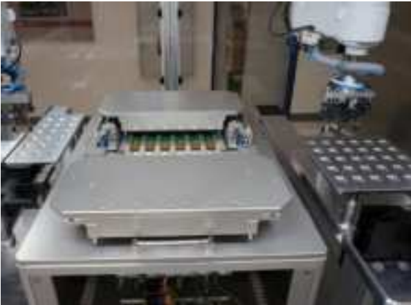
Figure 11: Automatic test equipment for module testing
