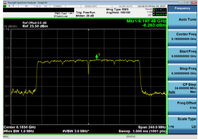
Plot 7-208. SP Power Spectral Density Plot Antenna WF7a (160MHz 802.11ax RU996x2 (UNII Band 5) – Ch. 47)
