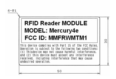
Measurements (unit: mm)
