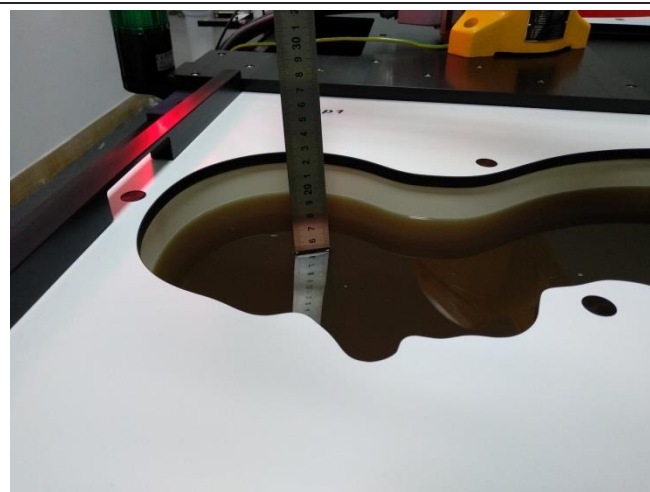
Liquid depth in the Head phantom
